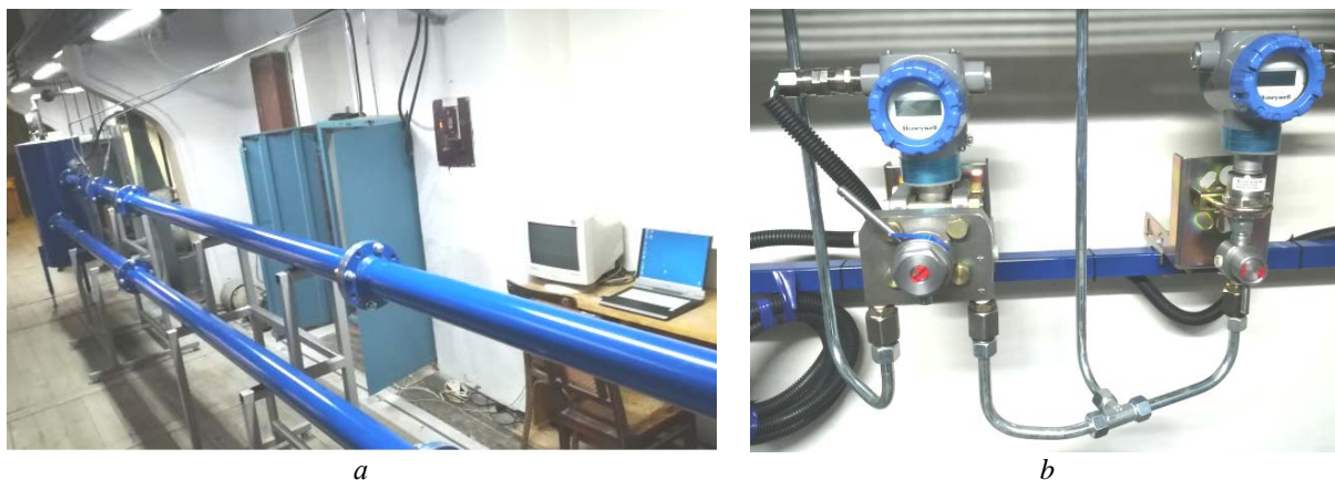
Fig. 1. Experimental setup: general view ( a ); panel with measuring transducers ( b )
