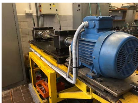
Fig. 2. Three-phase electric motor of Niemann M01
