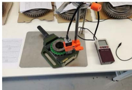
Fig. 4. Process of measuring of roughness by Mitutoyo SJ-201
