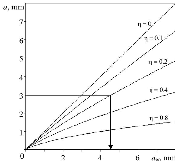
**Fig. 5.** Current sizes of defects depending on the initial size and number of loading cycles at  $\eta = N/[N_0]$
