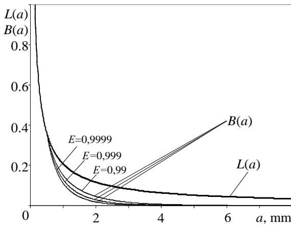
**Fig. 4.** Initial distribution of defects  $L(a)$  and distributions of defects after inspection  $B(a)$  with different efficiency
