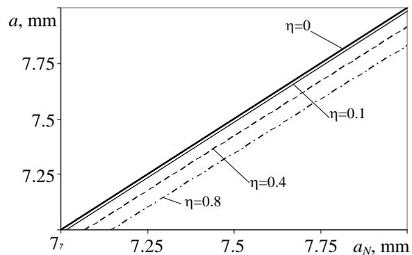
**Fig. 11.** Current sizes of defects depending on the initial size and number of loading cycles at  $\eta = N / [N_0]$
