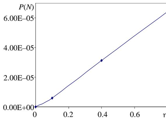
**Fig. 12.** Probability of pipeline failure during the period between inspections at different  $\eta = N/[N_0]$
