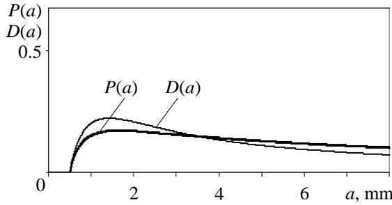
**Fig. 3.** Comparison of distributions of detected defects by their sizes based on calculated data  $D(a)$  and control experience  $P(a)$
