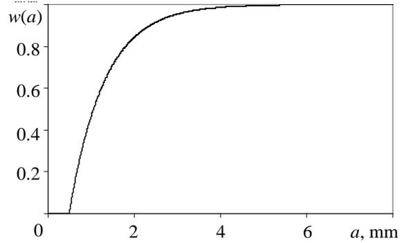
**Fig. 7.** Probability of detecting a defect depending on its size
