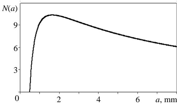
**Fig. 8.** Distribution of the number of detected defects for the emergency feedwater pipeline to the VVER-1000 steam generator
