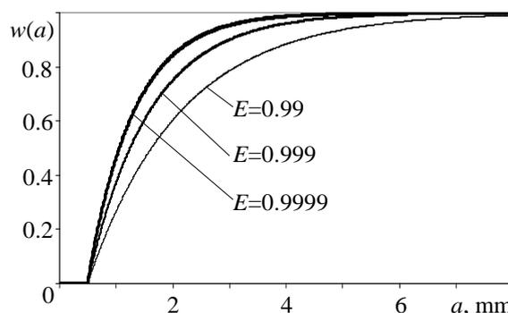
Fig. 2. Probability of detecting a defect depending on its size
