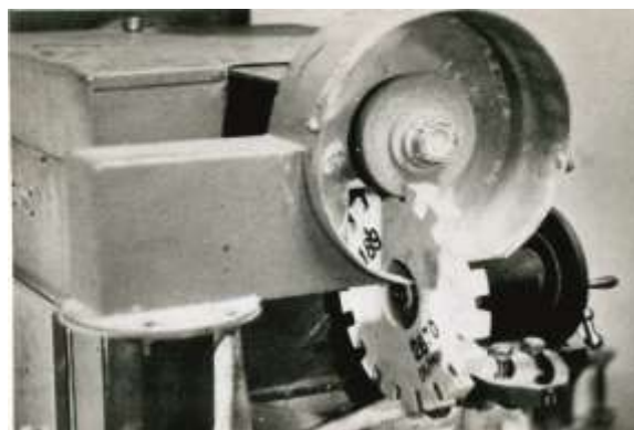
Fig.1. Cutting the grooves on the grinding wheel on the grinding machine
