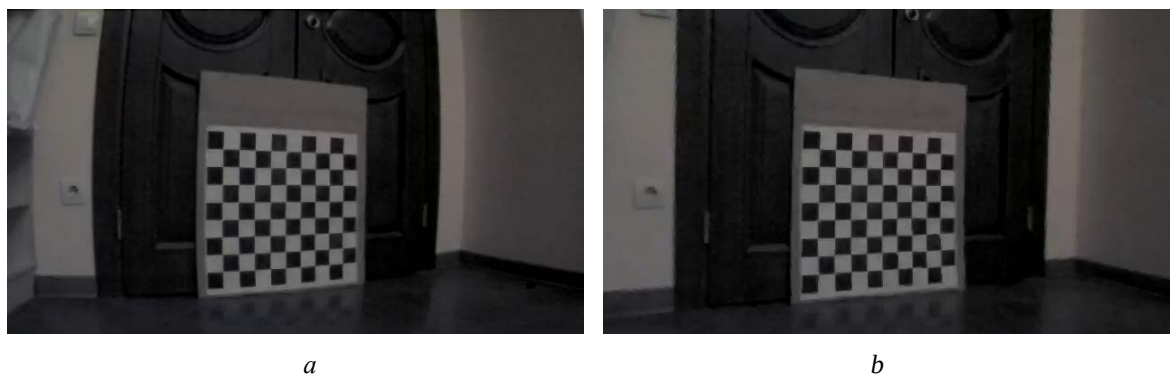
Fig. 7. Raw image from camera (a), undistorted image after camera calibration (b)
