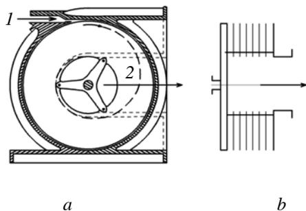
**Fig. 1.** Scheme of the Tesla disk turbine: *a* – side view; *b* – disks in section; 1 – steam inlet to the nozzle; 2 – steam
