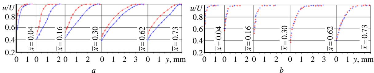
**Fig. 3.** Velocity plots in the boundary layer on the surface with  $x$  coordinate and flow modes with: at  $Re = 3.6 \cdot 10^5$  (o); at  $Re = 7.4 \cdot 10^5$  (+); *a* – surface roughness  $\bar{k} = 0.5 \cdot 10^{-3}$ ; *b* – smooth surface
