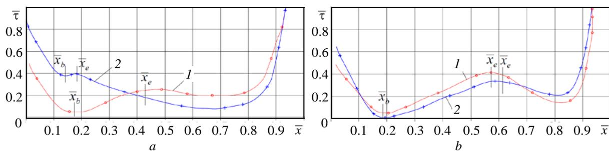
**Fig. 4.** Determination of the laminar flow zone in the boundary layer: 1 – at  $Re = 3.6 \cdot 10^5$ ; 2 – at  $Re = 7.4 \cdot 10^5$ ; *a* – surface roughness  $\bar{k} = 0.5 \cdot 10^{-3}$ ; *b* – smooth surface;  $\bar{x}_b$  – the beginning of the transition region,  $\bar{x}_e$  – the end of the transition region
