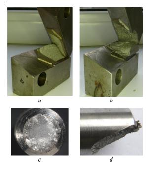
Fig. 5. Fractures of specimens: a, b – with an oblique incision modified compact; c, d – cylindrical. Test temperatures: 180 °C (a, c), –90 °C (b), +196 °C (d)
