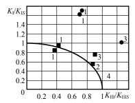
15Ch2NMFA(II) at different temperatures: - without PTL, - after PTL. Temperature: 1 - -196 °C; 2 - +180 °C; 3 - -90 °C; 4 - calculation by formula (8)
