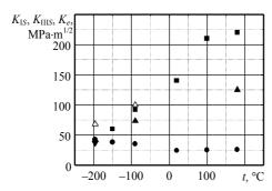
Fig. 6. Temperature dependence of fracture toughness:  $\blacksquare -K_{IS}$ ,  $\bullet -K_{IIIS}$ ,  $\blacktriangle -K_e$  (without preliminary thermomechanical load),  $\triangle -K_e$  (after preliminary thermomechanical load)
