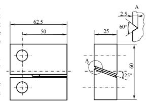
Fig. 1. Modified compact CT-1 sample with oblique fracture
