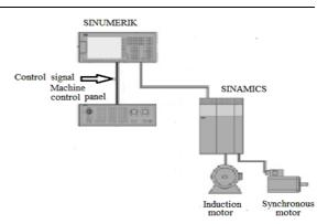
Fig. 2. The block diagram of control system with correction signal imitation
