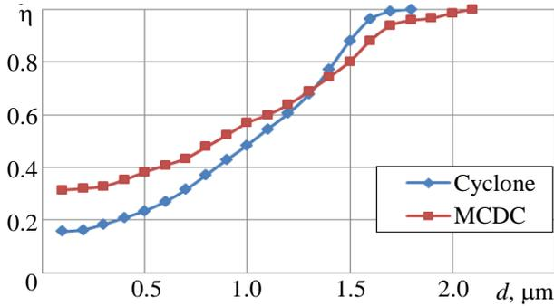
**Fig. 7.** Dependence of the capture coefficients by the cyclone and MCDC on the particle diameter
