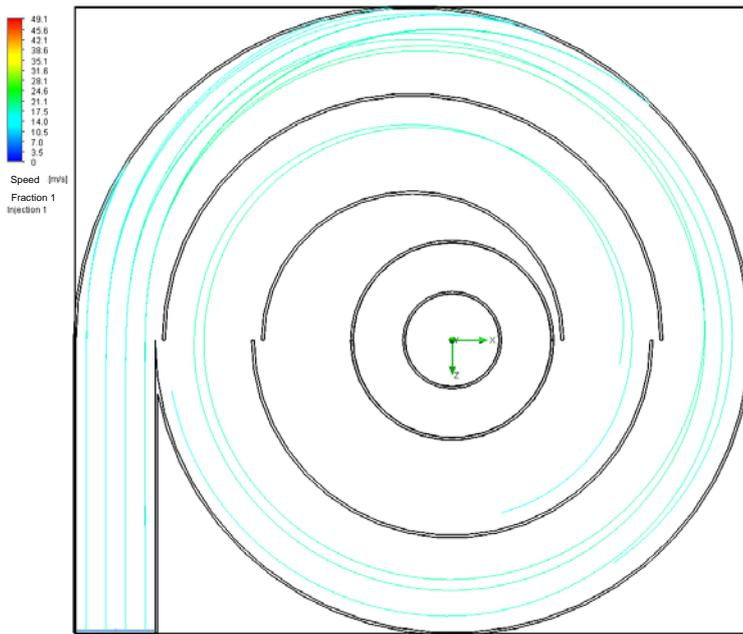
**Fig. 4.** Calculated trajectories of particles with a diameter of 9  $\mu\text{m}$  in the horizontal cross-sections of the MCDC
