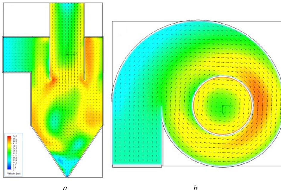
**Fig. 6.** Distribution of air velocities in the vertical (*a*) and horizontal (*b*) cross-sections of cyclone, obtained from the MCDC by discarding the outer half-shells
