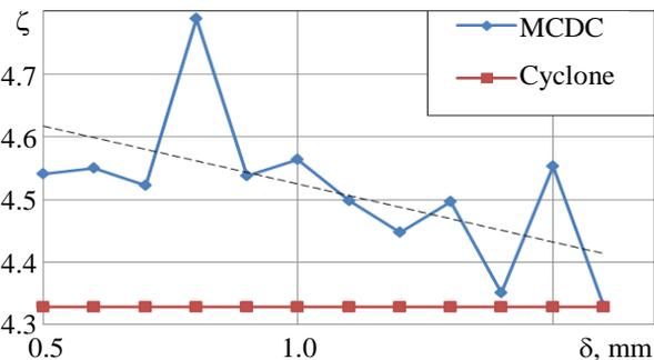
**Fig. 9.** Coefficient of hydraulic losses as a function of wall thickness
