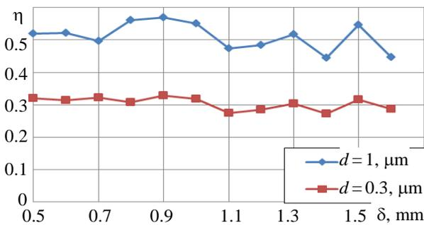
**Fig. 8.** Dependence of the coefficient of capture of particles with a diameter of  $d = 1 \mu\text{m}$  and  $d = 0.3 \mu\text{m}$  on the wall thickness
