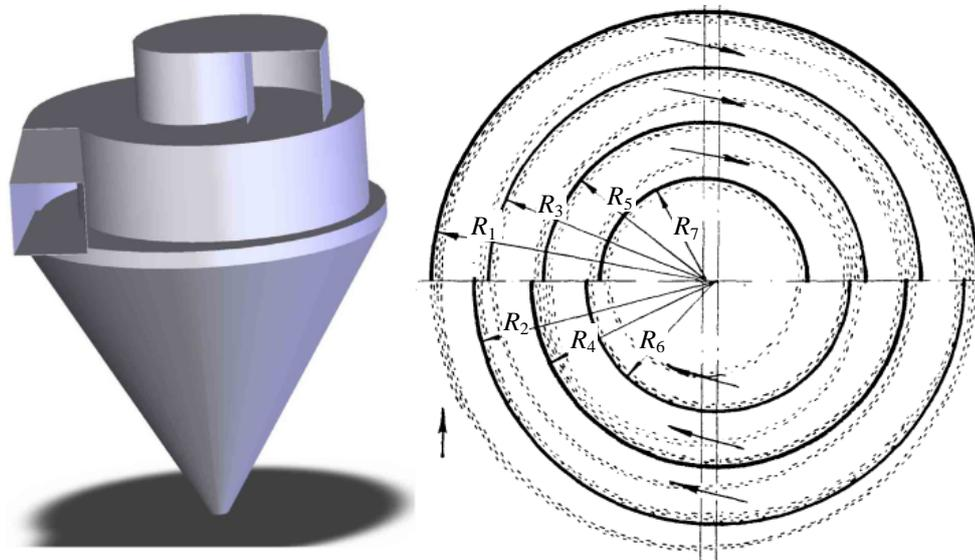
**Fig. 1.** General view of the MCDC and a diagram illustrating the proposed principle of its operation according to [2]
