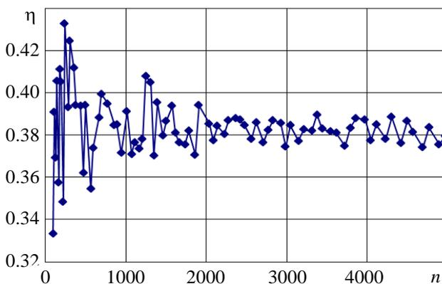
**Fig. 5.** Influence of the number of particles participating in the numerical experiment on the calculated capture coefficient  $\eta$  (diameter of the particles  $d = 0.5 \mu\text{m}$ )
