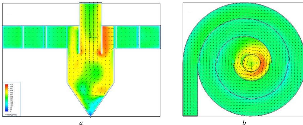
**Fig. 2.** Calculated distributions of air velocities in the vertical (*a*) and horizontal (*b*) cross-sections of the MCDC
