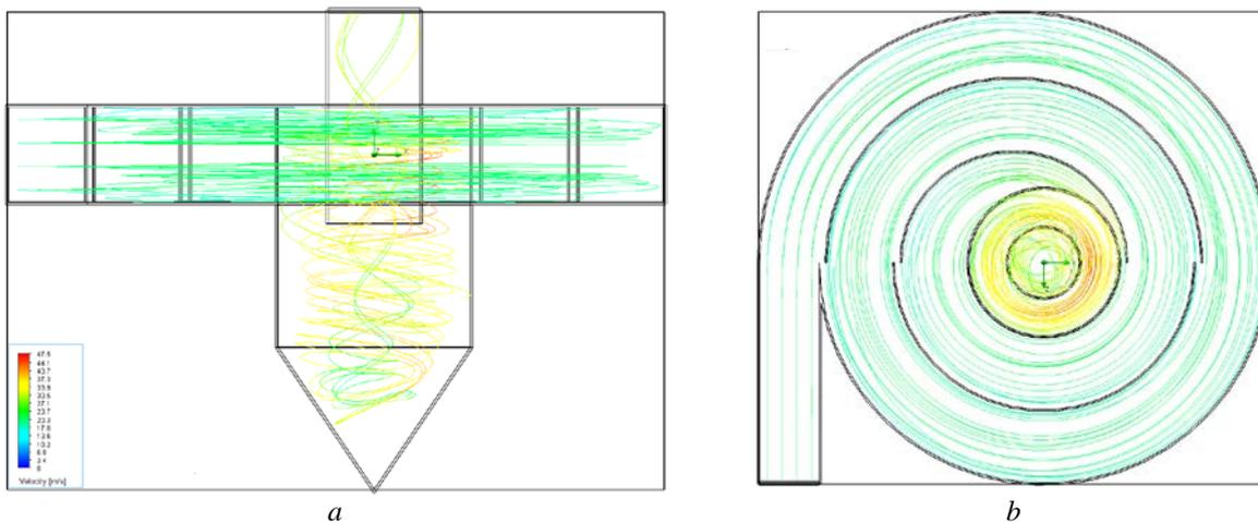
**Fig. 3.** Calculated trajectories of particles with a diameter of  $1 \mu\text{m}$  in the vertical (*a*) and horizontal (*b*) cross-sections of the MCDC
