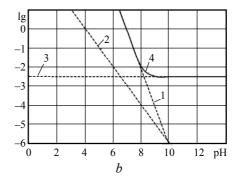
Fig. 1. Distribution dependence  $Co^{2^+}$  (1), cobalt hydroxo complex  $CoOH^+$  (2), cobalt hydroxide  $Co(OH)_2$  (3) and overall solubility (4) of the pH at: a - I = 0, b - I = 1
