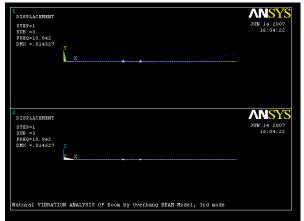
Fig. 18. Mode Shape of boom by beam model, 3<sup>rd</sup> mode
