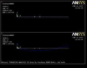
Fig. 16. Mode Shape of boom by beam model, 1<sup>st</sup> mode Fig. 17. Mode Shape of boom by beam model, 2<sup>nd</sup> mode
