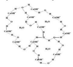
Fig. 5. Formation of clusters through hydrogen bonds
