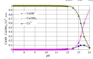
Fig. 4. Distribution of forms of existence of calcium compounds from solution pH upon reaching the thicken-
