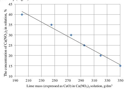
Fig. 2. Dependence of lime concentration in the transport solution on Ca(NO<sub>3</sub>)<sub>2</sub> concentration
