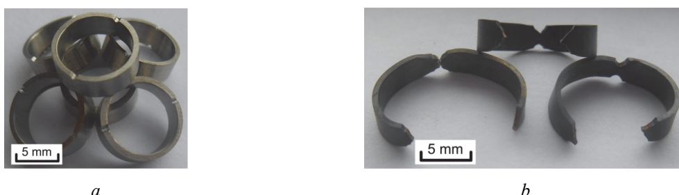
Fig. 7. General view of ring-samples of Zr-1 %Nb alloy rings during long-term static strength tests: before the tests (a), after the tests (b)
