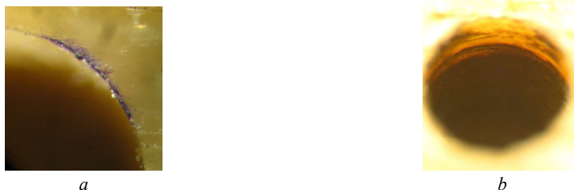
Fig. 6. Thermal degradation of hole edge (a) and hole surface (b) during drilling GFRP [17]
