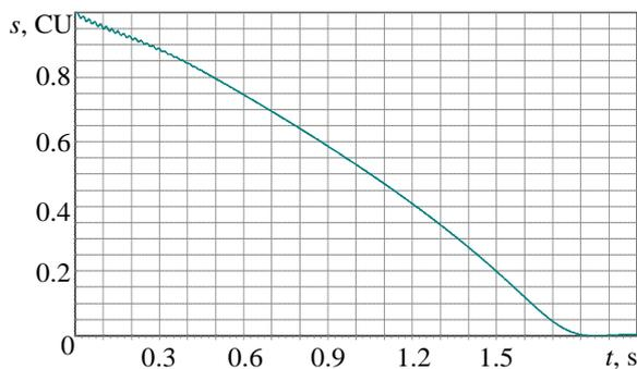
**Fig. 4.** The calculated curve of the slip change of IM with a capacity of 447 kW, a voltage of 6 kV at idle start-up
