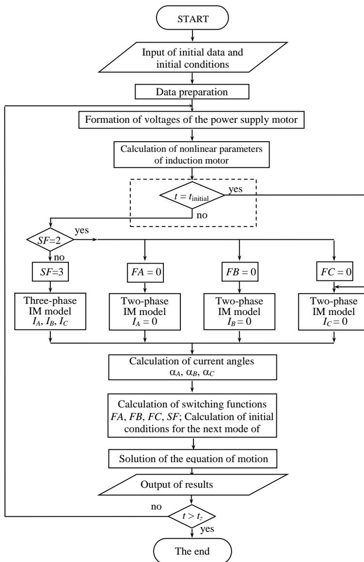
**Fig. 1.** Scheme of the IM simulation algorithm
