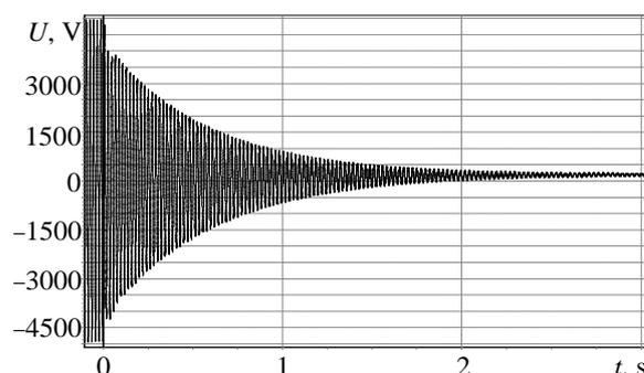
**Fig. 7.** Experimental curve of the change in the phase voltage of the IM stator winding with a power of 447 kW and a voltage of 6 kV at idle
