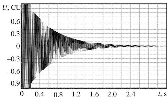
**Fig. 6.** Calculated curve of changes in the instantaneous relative values of the phase voltage of the IM stator winding with a power of 447 kW and a voltage of 6 kV at idle
