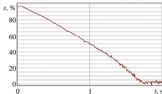
**Fig. 5.** Experimental curve of the slip change of IM with a capacity of 447 kW and a voltage of 6 kV at idle start-up
