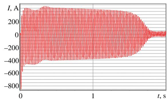
**Fig. 3.** Experimental curve of changes in the instantaneous values of the IM stator current with a power of 447 kW and a voltage of 6 kV during the idle start-up
