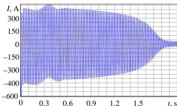
**Fig. 2.** The calculated curve of the change in the instantaneous values of the IM stator current with a capacity of 447 kW and a voltage of 6 kV during the idle start-up
