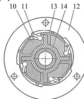
*Fig. 2. Structural scheme of blade turbine freewheel variance as an example of transmission implemented at the combined turbine drive assembly*
