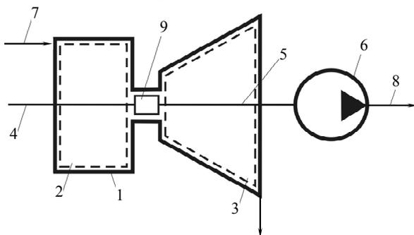
*Fig. 1. Scheme of two-rotors combined turbine drive with transmission for the NPP water supply emergency system pumping unit*
