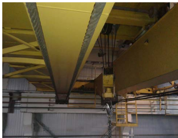
Fig. 1. Bridge crane with prestressed main beams
