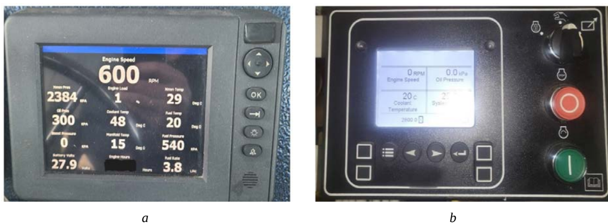
Fig. 2. On-board system for monitoring the operating parameters of the boat's powerplant: (a) multifunctional panel with color display; (b) control panel with digital display for the boat's engine
