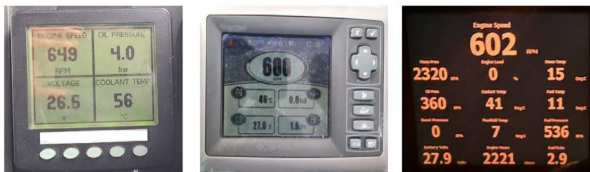
Fig. 1. Digital displays of the control and monitoring panel of the powerplant, which are installed on modern high-speed combat boats
