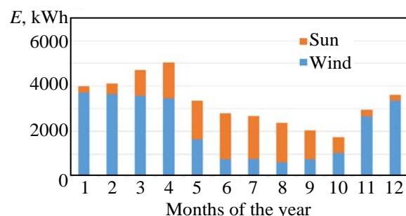
**Fig. 2.** Electricity generation by WPPs and SPPs by months of the year,  $V_{\text{av}} = 3.95 \text{ m/s}$
