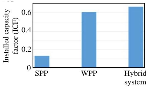
**Fig. 4.** Influence of the HSERES configuration on the installed capacity factor
