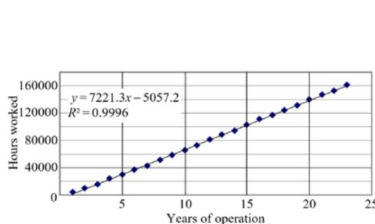
**Fig. 1.** Operating hours of power equipment in hours over years from commissioning
