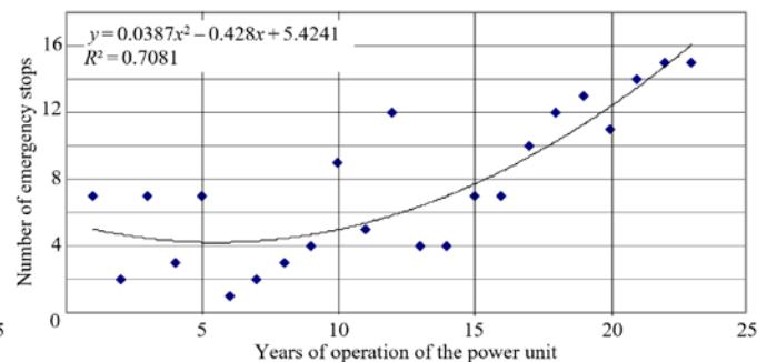
**Fig. 2.** Change in emergency shutdowns of the power unit over the years
