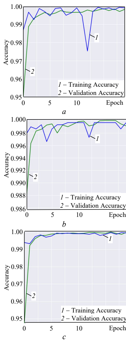
Fig. 7. Learning curves: a – for MLP; b – for MLP-KAN; c – for MLP-KAN-WT, showing both training and validation loss and accuracy over epochs
