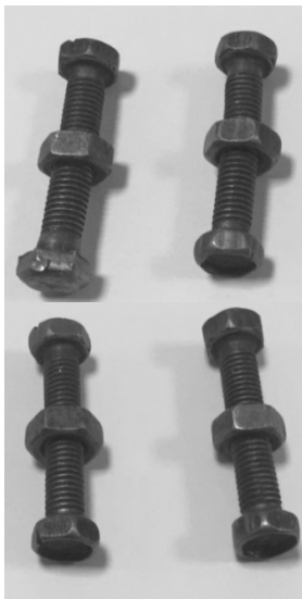
Fig. 1. Bolts are folded
