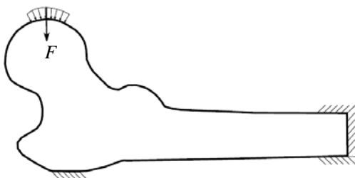
Fig. 3. Kinematic and force boundary conditions in the fall of man: F is the resulting force of the distributed load acting on the head of the femur
