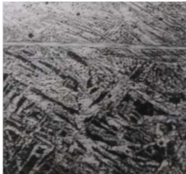
Fig. 5. The structure of the transition zone porous metal-ceramic shell – matrix
