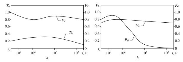
Fig. 3. MAMS with IAE "LOCA23 + blackout": maximum temperature of fuel claddings  $T_0$  and the coolant level in the reactor  $V_T(a)$ ; feedwater level  $V_L$  and pressure  $P_G$  in SG (b)
