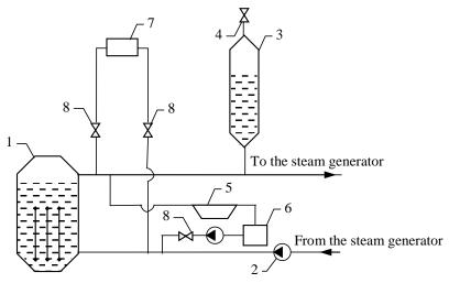
Fig. 1. ARPS R: 1 – reactor, 2 – main circulating pump (MCP), 3 – pressurizer, 4 – pressurizer safety valves, 5 – ARPS R1, 6 – hydraulic reservoirs of ECCS, 7 – ARPS R2, 8 – armature
